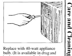
Replace with 40-watt appliance bulb. (It is available in drug and hardware stores.) Replace compartment cover. Plug in the oven.
